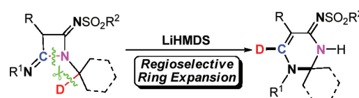
Scheme 1. Ring Expansion of 2,4-Diiminoazetidines via Cleavage of C–N and C(sp 3 )–H Bonds
